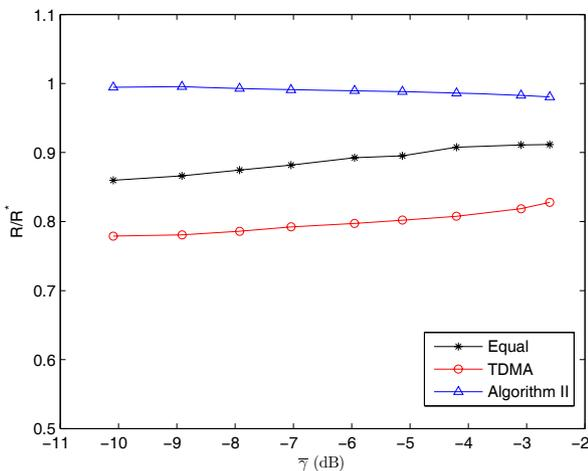
Fig. 2. Performance comparison in low SINR regions.  $d_{1,2} = 2$ ,  $\theta = 0.5$ ,  $Q = 2$ ,  $K = 2$ ,  $P_{S,i}^k = 1$ ,  $P_i^{\max} = 1$  and  $P_{i,k}^{\max} = 0.7$ , for  $i = 1, 2$  and  $k = 1, 2$ .  $R^*$  is the global optimal average sum rate and  $R$  is the average sum rate achieved by the proposed algorithm.
