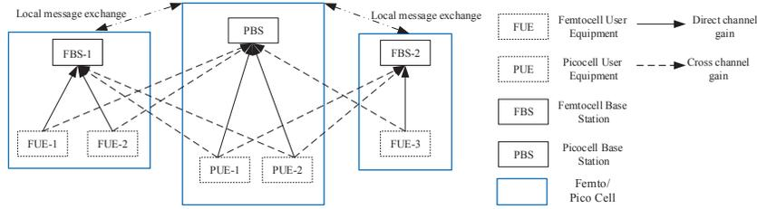
Figure 1. Illustration of a heterogeneous small cell network.
