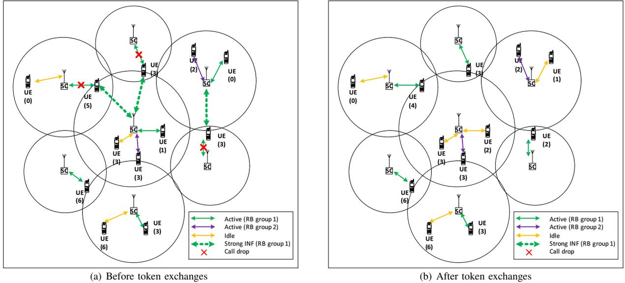
Fig. 1. Snapshot of a heterogeneous small cell network. The downlink interference problem is illustrated, (a) before and (b) after applying the token scheme. The number in the parentheses beneath “UE” indicates the number of tokens in its possession.
